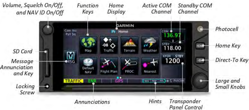
Figure 2 - GTN 635Xi/650Xi Control and Display Layout
