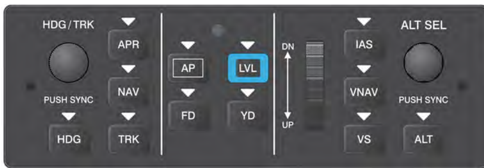
Figure 7-3: GMC 507 Control Unit (Reference Only)
