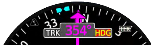
Figure 5- Top of the HSI when HDG failed (with GPS)
